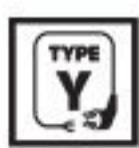
In the event that the power cable should become damaged, it should only be replaced by the manufacturer, its service facility or similarly qualified personnel.
